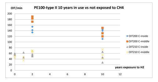
Figure 6. Oxygen induction time (OIT) versus years of hydrogen transport in the pilot hydrogen grid. A sample previously used in comparison to pipes previously not used.
