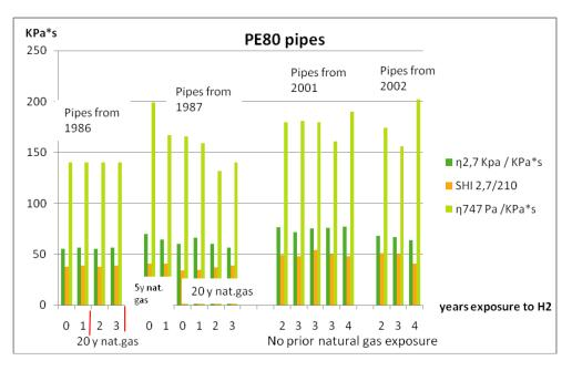
Figure 2. Rheological results of PE 80 pipes of different manufacturing years
