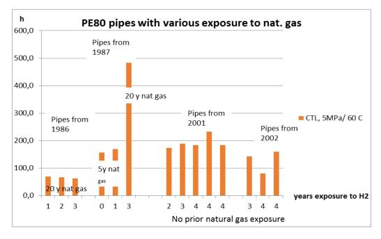
Figure 9. CTL resistance to slow crack growth of PE80 pipes of different manufacturing years
