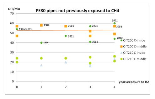
Figure 5. Oxygen Induction Time (OIT) versus years of hydrogen transport in the pilot hydrogen grid. Previously non-used pipes.
