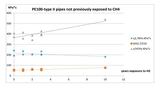
Figure 3. Rheology of PE 100 type II pipes, used for transportation of H<sub>2</sub> in the pilot grid, not previously exposed to CH<sub>4</sub>
