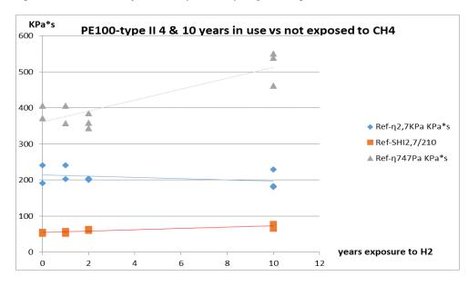
Figure 4. Rheology of PE100 type II pipes, used for transportation of  $H_2$  in the pilot grid compared to the combined effect of 4 years of natural gas transportation followed by 2 years of  $H_2$  transportation.
