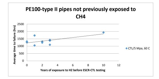
Figure 10. CTL resistance to slow crack growth of new PE100 pipes as a function of hydrogen exposure time
