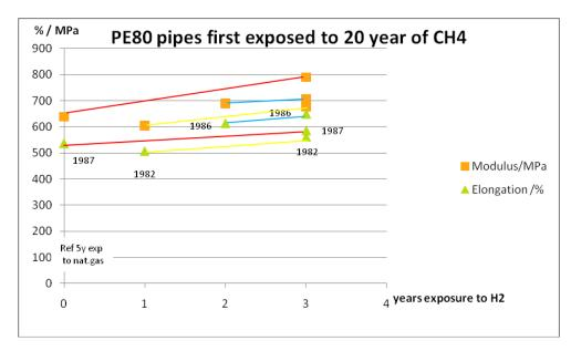
Figure 7. Elongation at break and tensile modulus versus years of exposure to hydrogen of pipes previously used for 20 years in the natural gas grid
